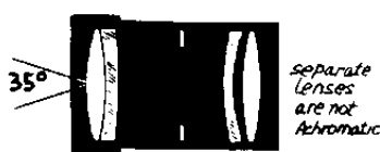
PETZVAL - f/4.5 BRIGHT AND SHARP AT CENTER BUT POOR AT EDGE
