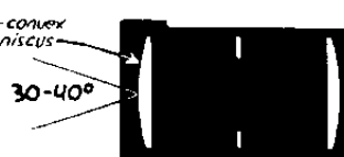
Simple Lens DUPLET - f/8 FAIRLY BRIGHT, FAIRLY SHARP-- THIS IS POPULAR HOMEMADE LENS
