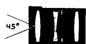
COOKE TRIPLET - f/3.5 BEST MEDIUM-PRICE LENS FOR EITHER CAMERA OR PROJECTOR
