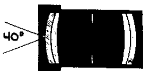
RAPID RECTILINEAR - f/8 THIS OLD-TIMER IS FAIRLY SHARP BUT DIM AT f/8
