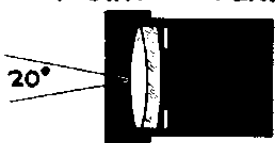
SINGLE ACHROMAT - f/4 USUAL NARROW-FIELD LENS IS FOR CAMERAS OR PROJECTORS
